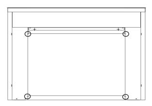
**NOTE:** When mounting the full screen door to the unit, the inside flange of the side trims are to fit over the inner side of the unit flange and <u>NOT</u> next to the outer side of the unit flange.
